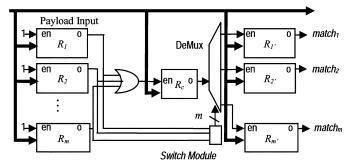
Fig. 5. Sharing architecture for infix and suffix.
