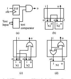
Fig. 8. Four basic NFA components [1]: (a) single-character; (b) concatenation; (c) union; (d) kleene-star.
