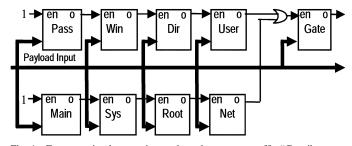
Fig. 4. Erroneous implementation to share the common suffix "Gate."
