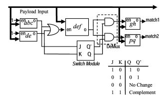
Fig. 7. Example of critical section problem.
