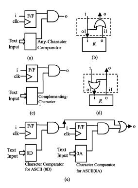
Fig. 9. New NFA components to support PCRE: (a) any-character matcher (.); (b) questionmark (?) quantifier (dashed box); (c) complemting-character () matcher; (d) plus quantifier (+) (dashed box).
